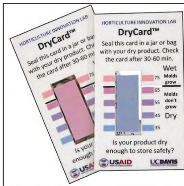
Fig. 7. The Horticulture Innovation Lab's DryCard. Pink means wet, not pink means dry.
