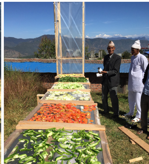
Built with widely available materials, the chimney solar dryer combines a table for drying fruits and vegetables with a chimney. Photos by Lauren Howe/UC Davis, 2018
