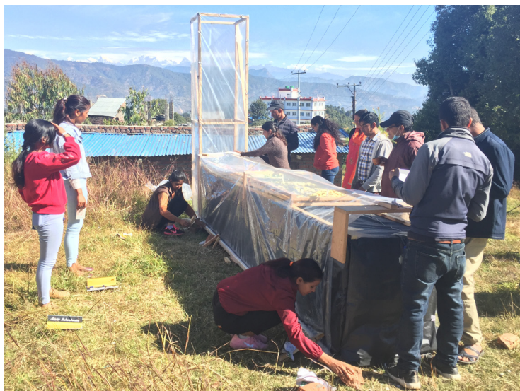
Built with widely available materials, the chimney solar dryer combines a table for drying fruits and vegetables with a chimney. Photos by Lauren Howe/UC Davis, 2018
