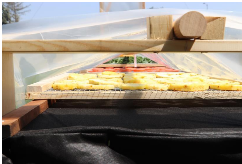
Figure 9. Only a few centimeters of headspace above the product, the plastic is not touching the product, and the front of the dryer is open. Note that trays can be stacked two high.
