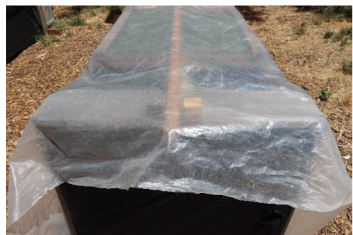
Make sure the wooden strips on the sides of the drying trays are not blocking the air from flowing over the product
