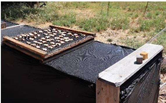
Align the wooden strips on the sides of the drying trays parallel with the sides of the drying table
