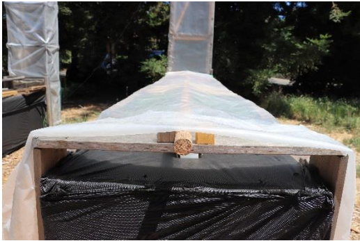
Figure 7. The front of the dryer is open for air to flow.
