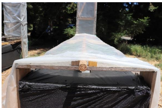
Align the wooden strips on the sides of the drying trays parallel with the sides of the drying table
