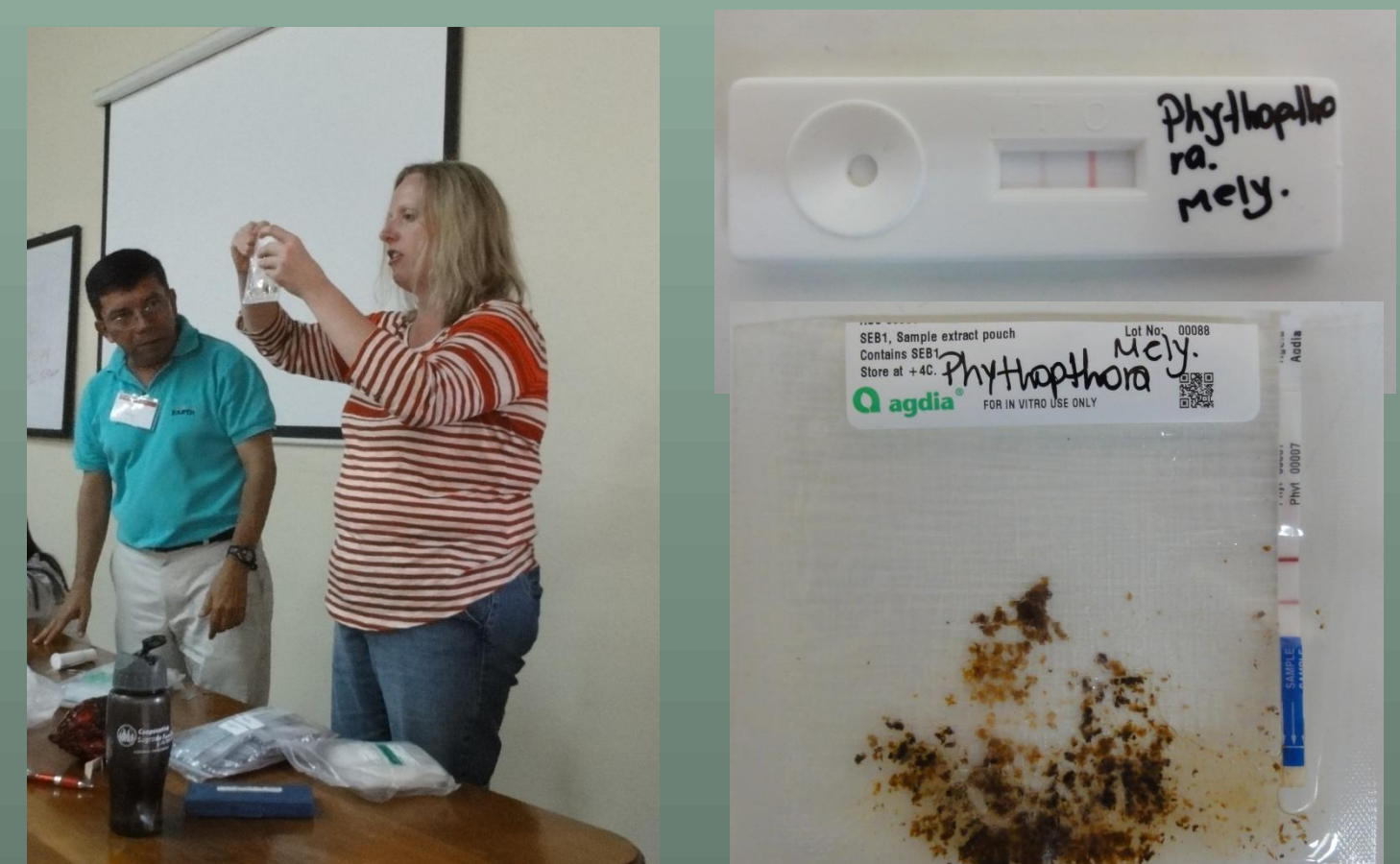
Fig 5. Instructors Jose Melgar and Kelly Ivors demonstrate the use of a rapid immunoassay kit for detecting Phytophthora .
